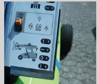
Multifunction control panel with integrated buttons and signal lights
